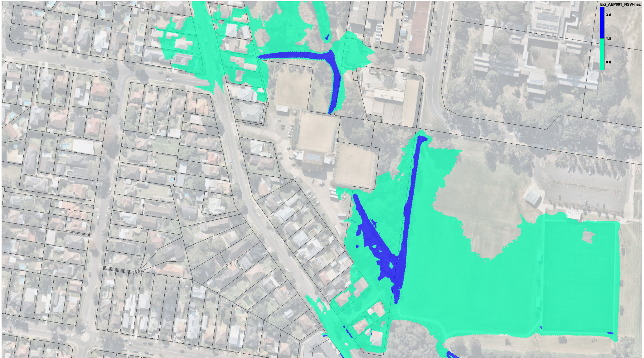
Figure A4: 1%AEP 30min Existing flood Hazard [NSW FDM] all-clear
